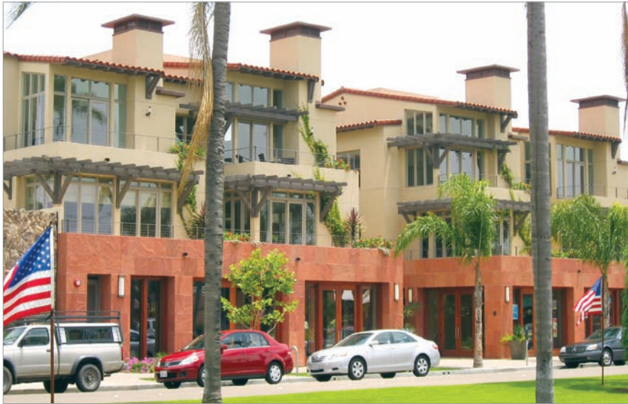
Dividing the horizontal elements of this building in Coronado helps it relate to its surroundings and the human scale.
