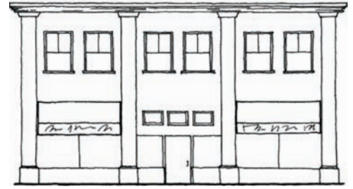
Vertical architectural elements subdivide the mass of a building into smaller increments.
