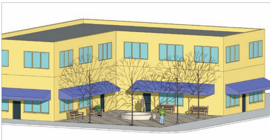
Deciduous trees allow for winter sun to penetrate into the plaza space.
