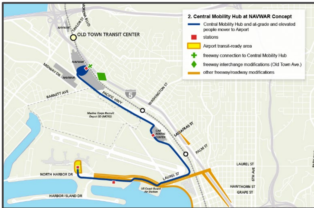
Figure Q-2. APM from SDIA to CMH at NAVWAR via At-Grade and Elevated
