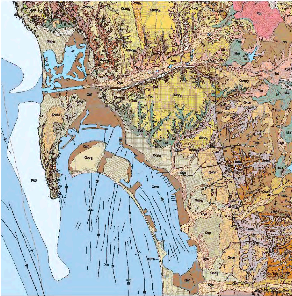
Figure 6 – Reclaimed Public Trust Tidelands are shown in the color Brown as Quaternary Artificial Fill (Qaf).
